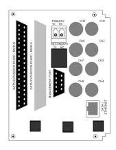
The AMG3708BRN-DR-SF is a rackmount data receive unit designed to receive to transmit and receive 9 bi-directional data channels to/from up to 8 AMG3703B2-DR-SF or AMG3703B2R-DR-SF rackmount equivalent insert units over a dual redundant singlemode optical fibre ring. One data channel is a multi-drop RS-485 link, the other eight data channels are effectivly point to point RS-232 links.
