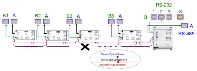
If multiple breaks occur, operation is maintained will all the units still physically connected to the receiver. For the scenario shown below data would now be lost from units 1 and 2 as there is now no physical connection between the transceivers and the receiver. However operation of units 3 and 4 to 8 remain fully functional.
